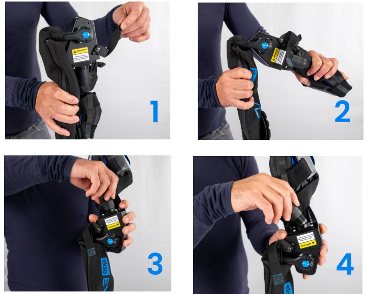
Figure 18: Installing Actuator Springs
