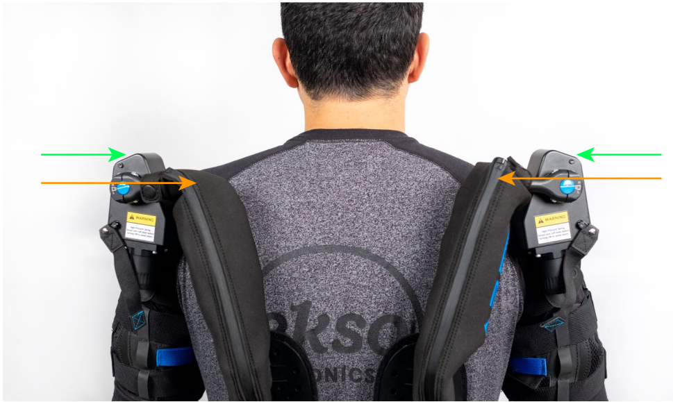
Figure 10: Proper Ekso EVO Actuator Height Alignment
