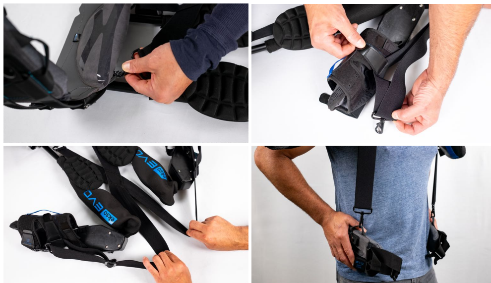
Figure 13: Installing Ekso EVO Suspenders
