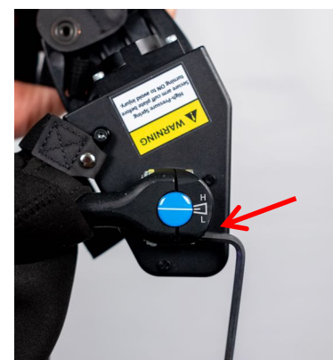
Figure 20: Loosening End Link Screw
